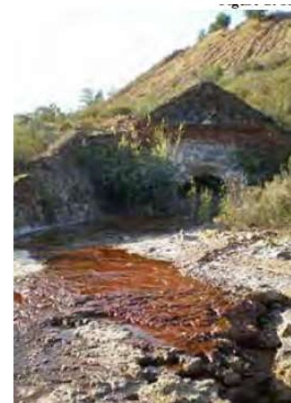
Figure 1. Roman Portal with Acid Rock Drainage – Spain INAP, The international Network for Acid Prevention (2014)
